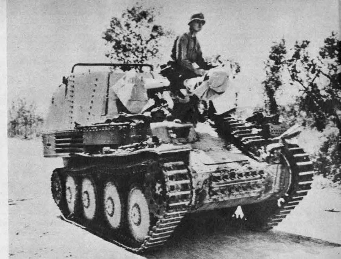
This captured Czech PzKw 38 chassis that mounts a 75-mm. is a favorite Nazi self-propelled weapon. The gun is housed in a tall, open-topped, slant-sided shield well to the rear.
